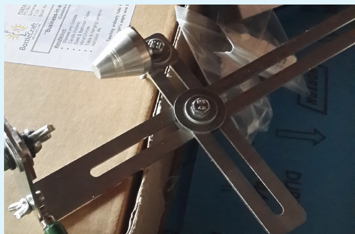
Artisanal glass cutting kit that is being used with waste glass from the tourism establishments in the TBT area, Mozambique (Photo: COAST Project)
